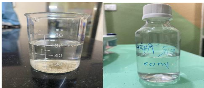
After 12 hours kankshi is Dissolved and some remaining Particles settle down and later the Solution is filtered.
