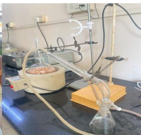
Extraction of Gulab Arka by Simple Distillation
