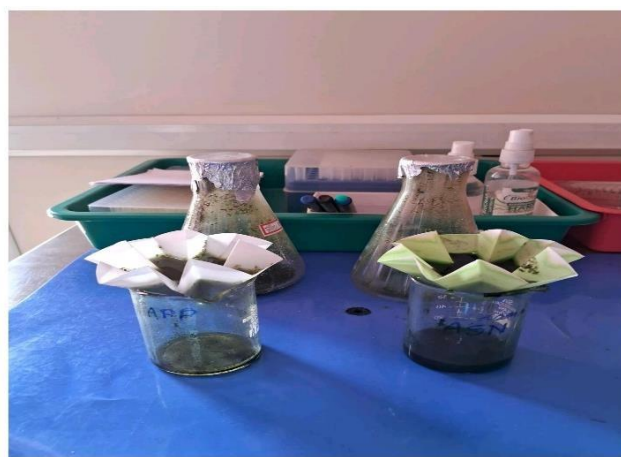
Fig. 1b: Filtration of the solvent extract.
