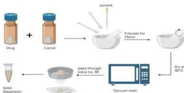
Fig.2.2: Schematic representation of Solid dispersion preparation by Kneading method.
