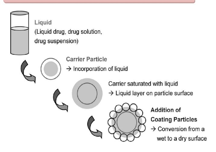
Fig. 1: Schematic representation of liquisolid systems<sup>[23]</sup>
