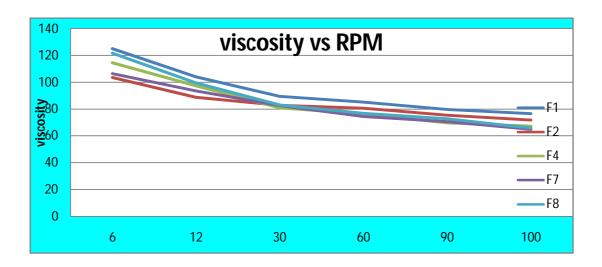
"Fig. 3" Viscosity graph of microemulsions.
