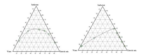
"Fig. 1" The ternary phase diagrams of eutectic mixture, tween 80 and water in presence and absence of co-surfactant (ethanol); (a) co-surfactant free system,(b) 1:1 ratio of tween 80 and ethanol,(c) 1:2 ratio of tween 80 and ethanol, (d) 2:1 ratio of tween 80 and ethanol.
