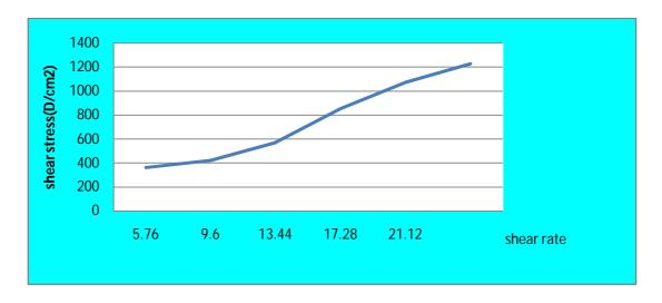
Fig. 7 Graph between shear rate and shear stress of hydrogel.
