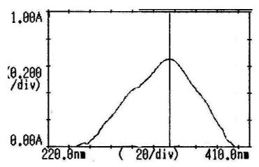
Fig no 1 Nimodipine in Methanol at 346 nm
