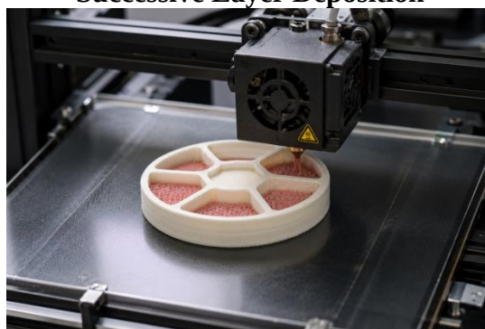
Fig 1: Fused Deposition Modelling (FDM)
