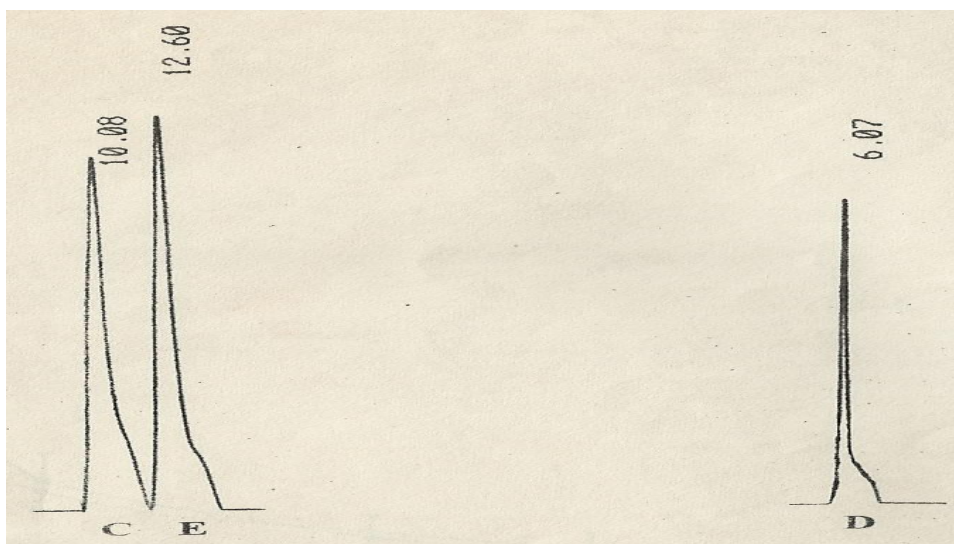
Fig. 1: Representative HPLC chromatogram obtained from dual wavelength UV detector at 278 nm (enrofloxacin and ciprofloxacin) and at 280 nm (diclofenac)
