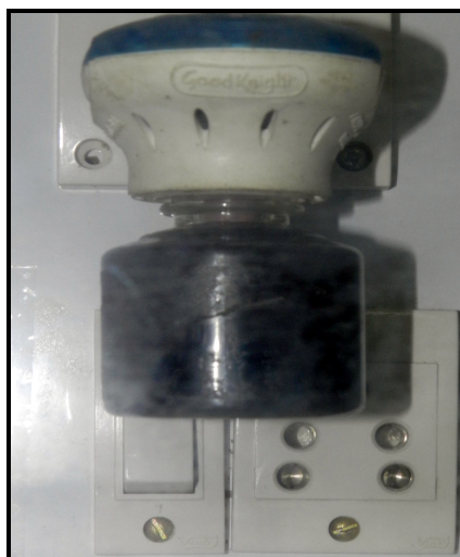
Figure 1 Electrical vaporizer container of biopesticide Repellent solution
