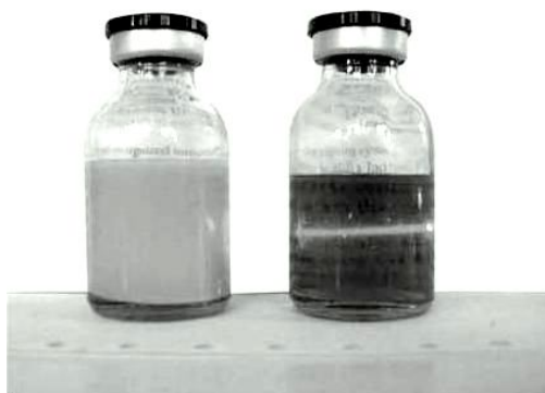
FIGURE 8 Two nanosuspensions composed similarly, produced by high-pressure homogenization, conventional method (left) versus translucent nanosuspension (particle size well below 100 nm) resulting from H96 technology. The red laser beam is reflected by the tiny nanocrystals.
