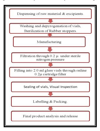
Fig.: Process flow diagram of parenteral dosage form
