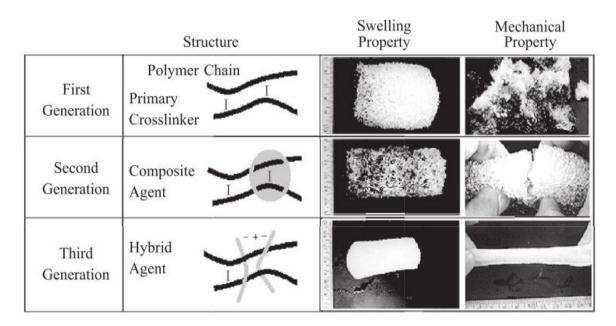
Fig. 2 Structural, Swelling and Mechanical Properties of Different Generations of SPHs.
