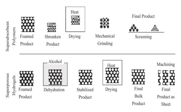
Fig. 4 Post-synthesis steps of SAPs and SPHs.
