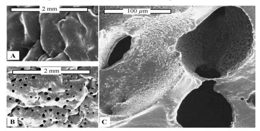
Fig.1. Scanning Electron Micrographs of a Nonporous SAP (A) and a Corresponding SPH (B and C).
