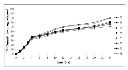
Fig. 2: Comparative in-vitro release profiles of Selegiline hydrochloride proniosome gel formulations in pH 7.4 buffer.
