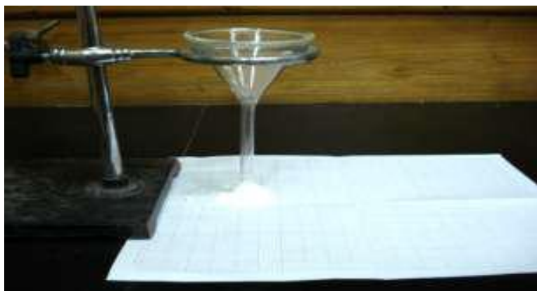
Figure: Measurement of angle of repose (Fixed Funnel method).
