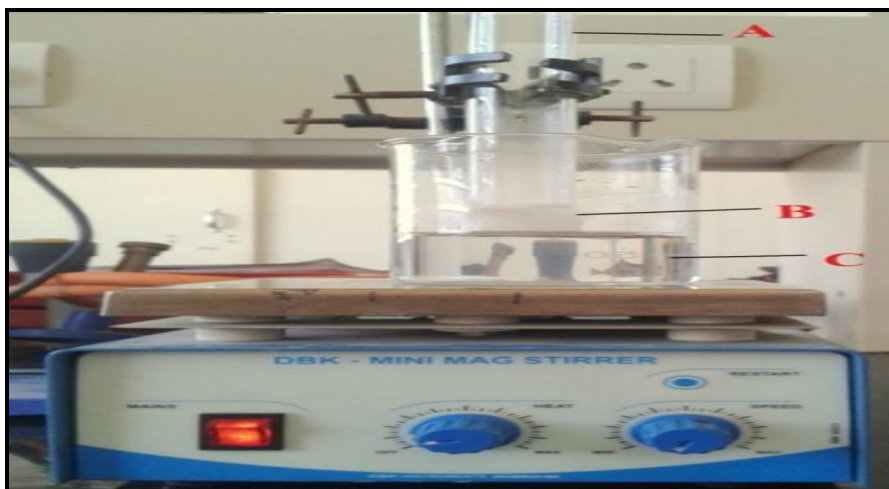
Figure 6. Laboratory designed diffusion cell A- Tube containing formulation, B- Egg membrane, and C- Beaker containing simulated tear fluid.
