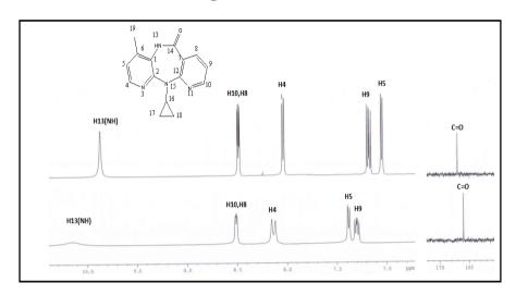
Fig.10 NMR spectra of nevirapine [200  $\mu M]$  in absence and presence of BSA [25  $\mu M]$  at 298 K
