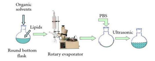
Fig-3: Preparation of Liposomes using Rotary Evaporator.
