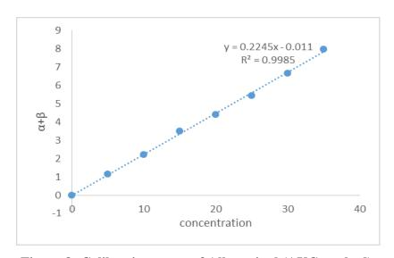
Figure 8: Calibration curve of Allopurinol (AUC method).
