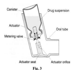
Pressurized aerosols may be formulated as either solutions or suspensions of drug in the liquefied propellant. Solution preparations are two-phase systems. However, the propellants are poor solvents for most drugs. Cosolvents such as ethanol or isopropanol may be used,
