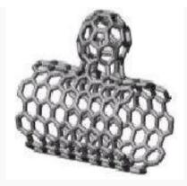
In theory, a nanotorus is a carbon nanotube bent into a torus (doughnut shape). Nanotori are predicted to have many unique properties, such as magnetic moments 1000 times larger than previously expected for certain specific radii. Properties such as magnetic moment, thermal stability, etc. vary widely depending on radius of the torus and radius of the tube.
