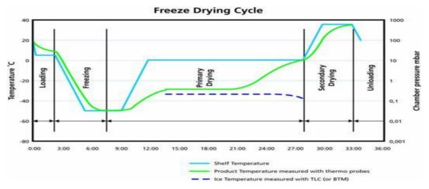
Fig: A typical freeze drying cycle showing shelf temperature, product temperature on different time under pressure in mbar.
