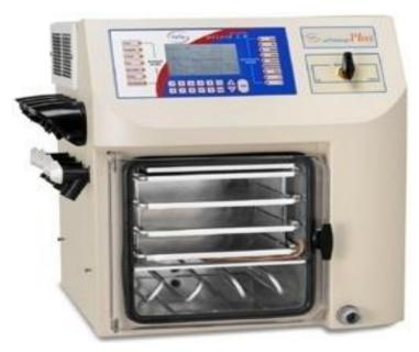
Fig: A benchtop freeze dryer, front view<sup>[14]</sup>.
