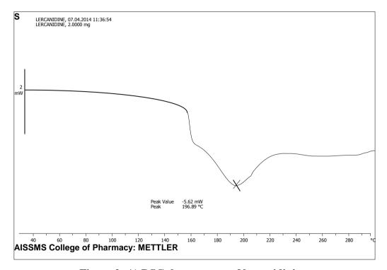
Figure 2: A) DSC thermogram of lercanidipine.
