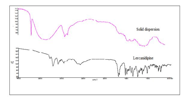
Fig. 1: IR Specta of Pure Lercanidipine and Solid dispersion.
