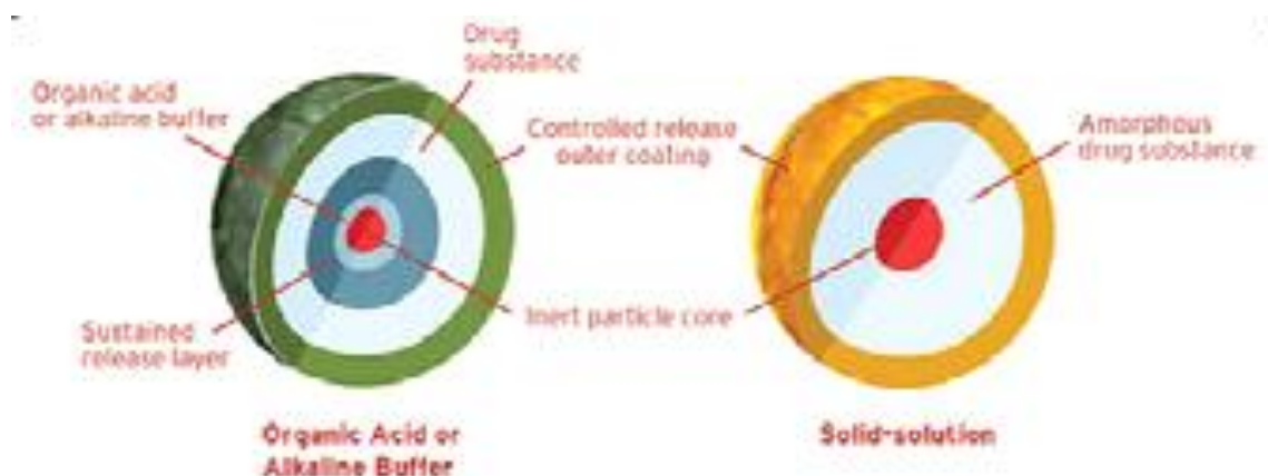
Fig. 11: DIFFUCAPS bead surrounded by organic acid or alkaline buffer layer
