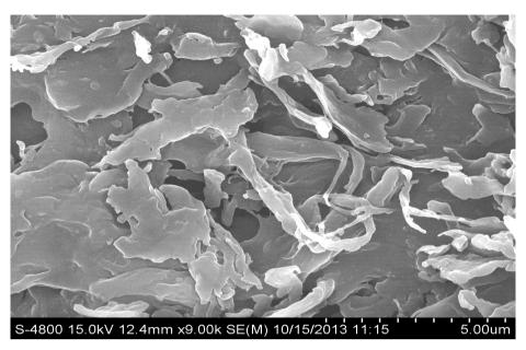
Fig: 3 SEM image of Chitosan-g-MAN composite
