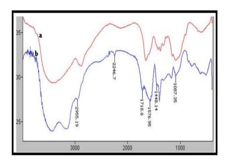
Fig. 2 – IR Spectra of a) Chitosan B) Chitosan-g- methacrylonitrile
