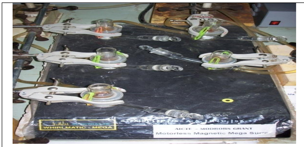
Fig 13: Experimental set up for in vitro permeation studies
