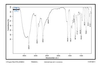
Figure1: FTIR spectrum of Tramadol Hcl
