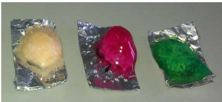
Fig. 6 Pictures of tablets prepared from pellets via three-stage extrusion, taken at 5 h of dissolution study: yellow – E1-3, red – E2-3 and green- E3-3.
