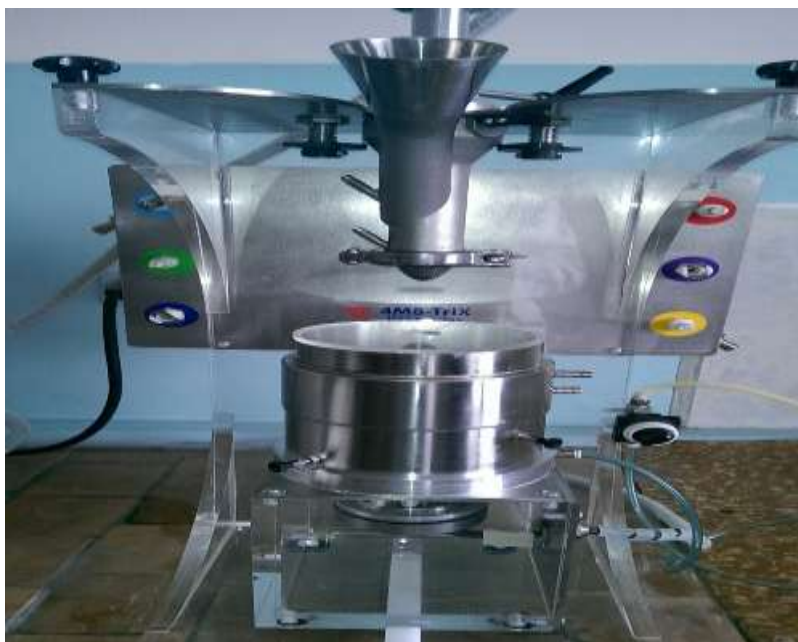
Fig. 2 Radial screw-feed extruder (4M8Trix, Procept, Belgium)
