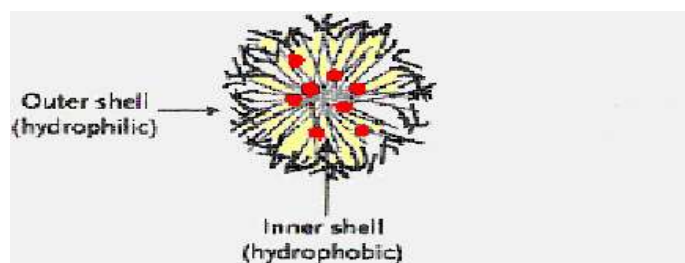
Fig. 3: Cross Section of polymeric micelles. [29]
