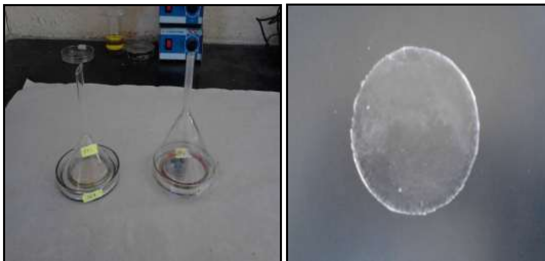
“Fig.1: Formulation of Ondansetron hydrochloride and Diltiazem hydrochloride film on mercury surface with glass ring mould.”
