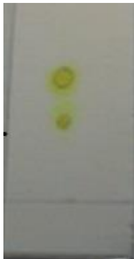
Fig. 5 Thin layer chromatography of D-pinitol
