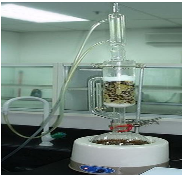
Fig1: A picture of Soxhlet apparatus during an extraction
