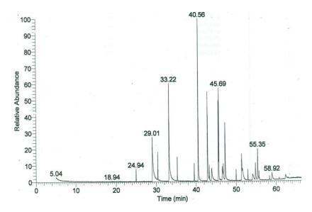
Figure 1.The retention time (min) versus the relative abundance of 6 phthalates by GC-MS. Injected volume 1 ul containing 25 ng, each of DMP, DEP, DBP, BBP, DEHP & DOP.
