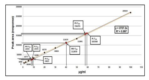
Fig 1: Standard curve for total and soluble oxalic acid contents.
