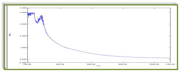
Figure (4): UV absorbance of extracted pyomelanin pigment.
