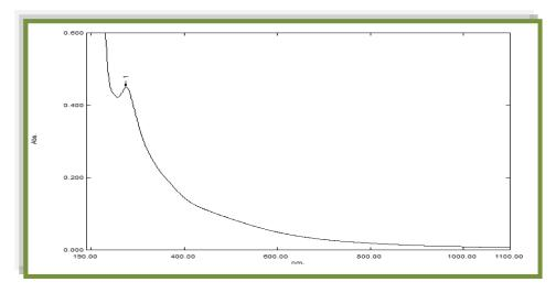
Figure (3): UV absorbance of synthetic pyomelanin pigment.
