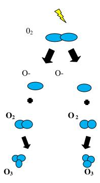
An electrical discharge splits an O2 molecule into two oxygen atoms (electrical discharge also referred to as corona discharge). These unstable O2 atoms combine with each other oxygen molecules. This combination forms ozone.
