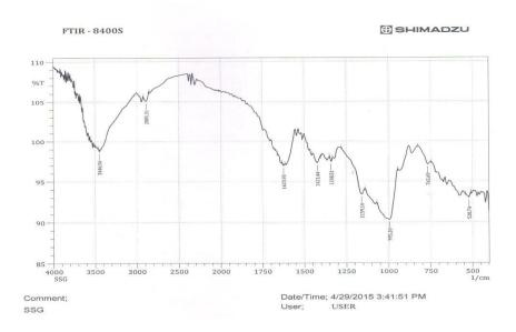
Fig 2: FT – IR Spectrum of Sodium Starch Glycolate
