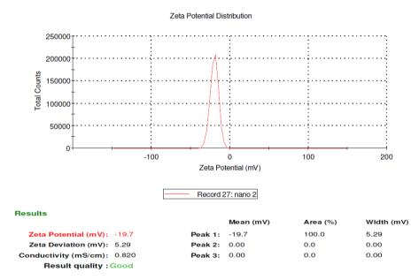
Zeta Potential (mV): from  $\pm 10$  to  $\pm 30$  = Incipient instability Figure 6. Zeta Potential Measurement of Au Nanoparticles
