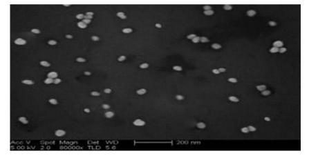
Figure 4. SEM -microscopic view of A. vasica reduced gold nano particles.
