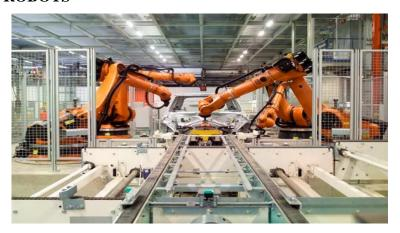
"An automatically controlled, reprogrammable, multipurpose manipulators which may be either fixed in place or mobile for use in industrial automation applications." The kinds of robots which form the most commonly used industrial robots are robots with fixed arms ands manipulators chiefly doing work related to production and distribution of goods.
