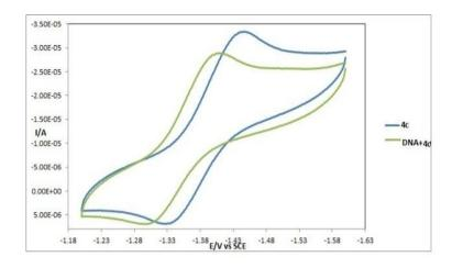
Figure 7: Cyclic Voltammogram for (0.1M) B at Scan Rate of 0.2V/s in Ethanol Water Mixture (8:2) at pH 7.4.
