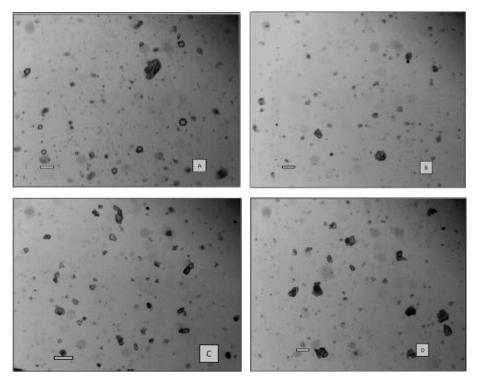
Figures 1 (A-D). Photomicrographs of representative batches of microparticles: A, B, C, and D contain 200, 300, 400 and 0 mg of ibuprofen, respectively. Bar represents various sizes in  $\mu$ m.
