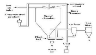
Figure 7: Spray Drying Method for Preparation of Microsphere
