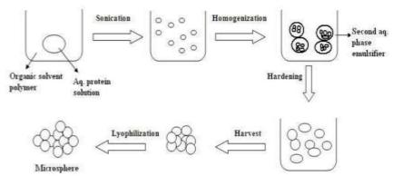
Figure 8: Solvent Evaporation Method For Preparation of Microsphere
