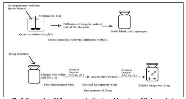
Fig. 3: Preparation of Microsponges by Quasi-emulsion solvent diffusion method.
