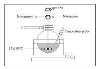
Fig. 2: Reaction vessel for Microsponge preparation by liquid-liquid suspension polymerization.
