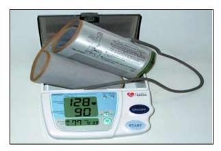
Fig 2: A digital blood pressure meter
