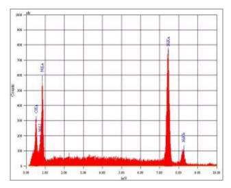
Fig 6: EDS spectrum of NiO nanoparticles and composition of elements.
