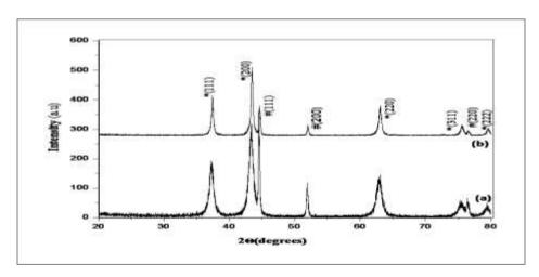
Figure 4: Shows X-ray diffraction pattern of prepared nickel nanoparticles. (a)TBAB (b) TOAB at 10mA/cm.<sup>2</sup>
