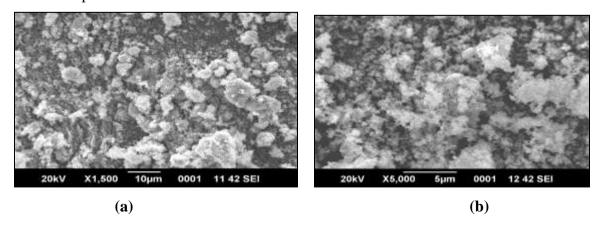
Figure 5: shows SEM image of nickel nanoparticles: 1500 and 5000 magnification with (a) TBAB (b) TOAB at 10mA/cm<sup>2</sup>.
