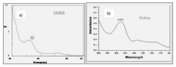
Fig. 3 Optical absorption spectrum for Ni nanoparticles (a) TBAB and (b) TOAB at current density 10mA/cm<sup>2</sup>.
