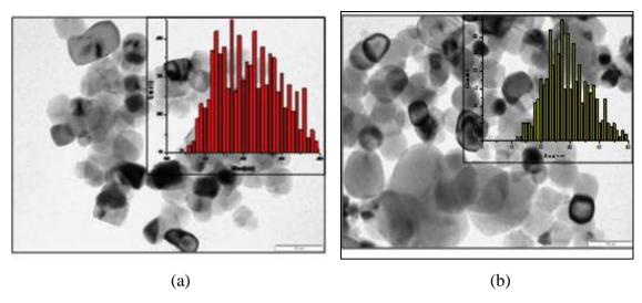
Figure 7: Shows TEM image of nickel nanoparticles and histogram at (a) TBAB (b) TOAB at 10mA/cm<sup>2</sup>.
