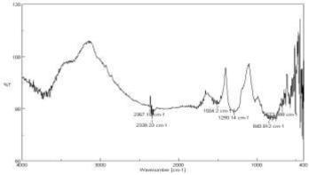
Fig 3. FTIR spectrum of silver nanoparticles generated by PDB
