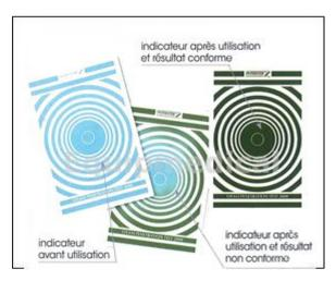
Several assumptions are challenged whenever an unsatisfactory test of the turn is found or the clear and objective interpretation does not carry out: the performance of the autoclave itself, expiration and conditions conservation of this test in the structures of use?.
