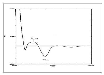
Fig. 2 difference absorption spectra of basic solution of bupropion against acidic solution.
