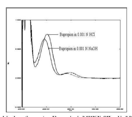
Fig.1 overlain absorption spectra of bupropion in 0.001N NaOH and in 0.001N HCl.
