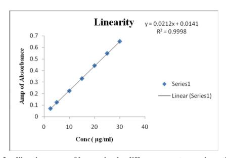
Fig 3 calibration curve of bupropion by difference spectroscopic method
