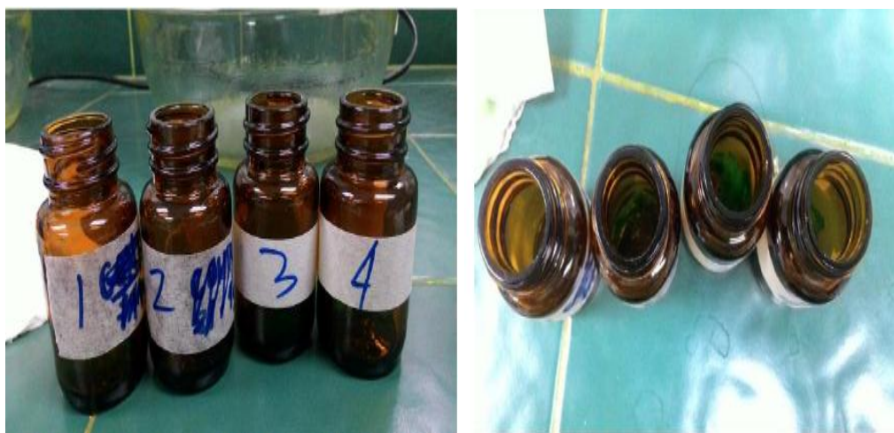
Figure: 10 Subjecting of the films to anhydrous calcium chloride maintained in the same container.
