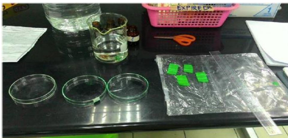
Figure 9. Preparation of the films for linear expansion coefficient testing in water
