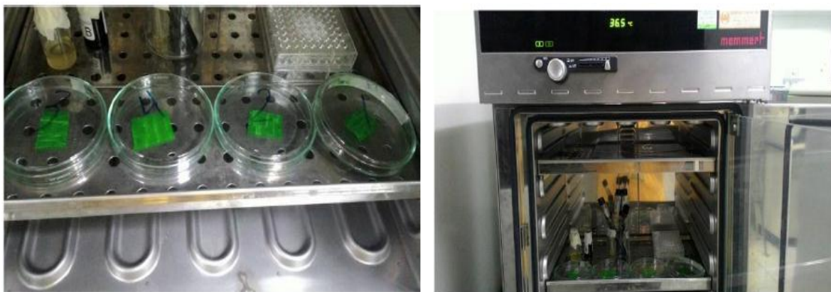
Figure 8. The films subjected to swelling in a petri dish and left in the Memmert oven.
