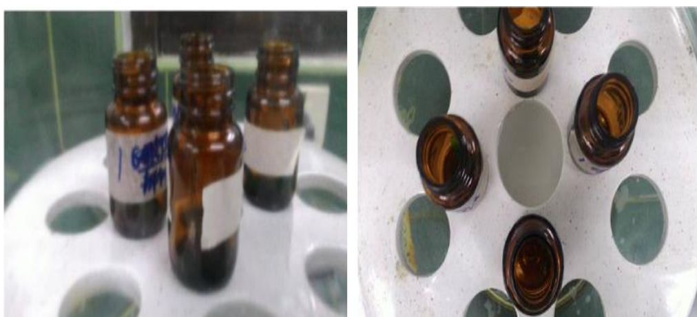
Figure 11. Leaving of the films inside the dessicator for 72 hours.
