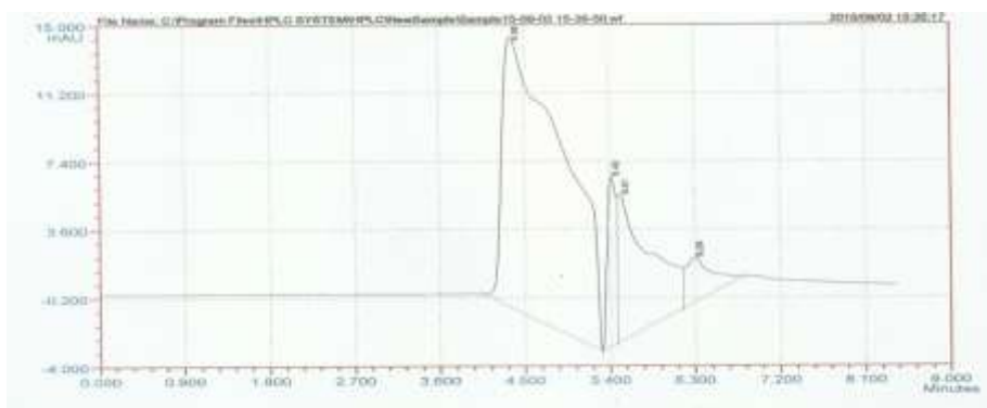
Fig. 5: Chromatogram after injection of 60 µg/ml of artesunate and amodiaquine.
