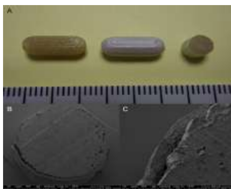
Fig.1. Images of 3DP fabricated caplets (A) from left to right, caplet prior to coating, caplet after coating and cross section of coated caplet (scale in cm); (B, C) SEM images of internal structure of cross-section of a coated-3D printed caplet. [16]
